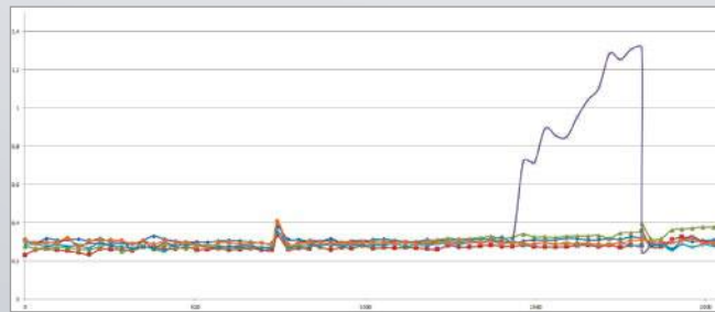
Six movers in online monitoring: the impending failure of a ball bearing shows several days in advance.
