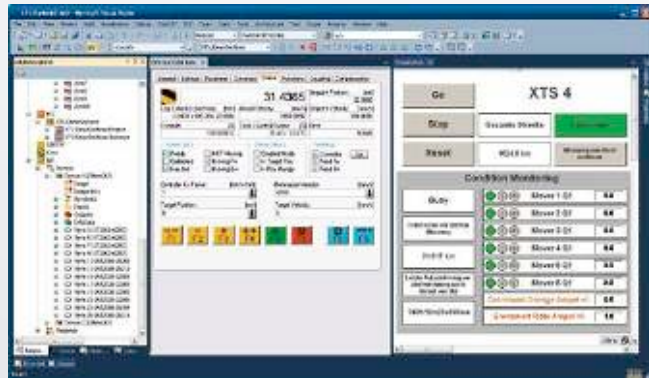
The information from the Condition Monitoring can be reduced and simplified to a "traffic light"-style status display.
